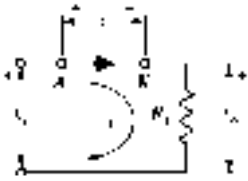
Fig. 4-1 The basic diode circuit. The anode (the p side) of the diode is marked A , and the cathode (the n side) is labeled K .
