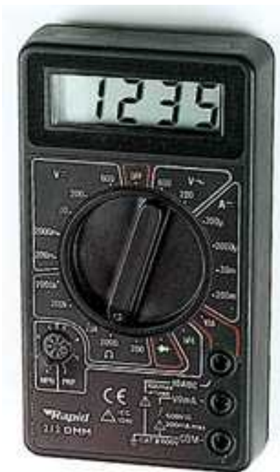
EXAMPLE OF DIGITAL METER
