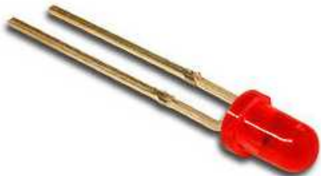
ENLARGED LED - NOTICE THE LONG AND SHORT LEG
